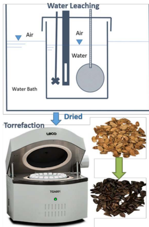
Figure 12. Laboratory scale leaching and torrefaction test equipment.
