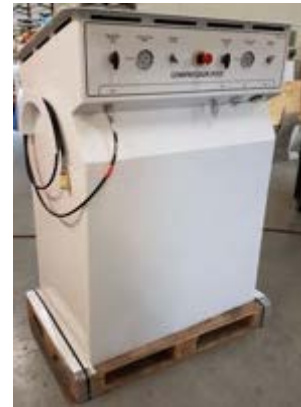
Figure 7. MTA boost compressor fueling post.
