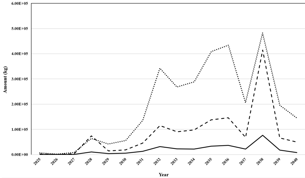
Figure 41. Aggregate metals loading from ancillary components at all scale in Maui County. Legend: Copper (solid line), aluminum (dashed line), and steel (dotted line).
