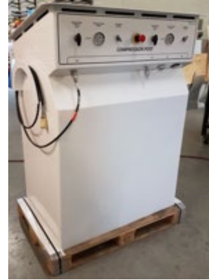
Figure 7. MTA Boost Compressor Fueling Post.
