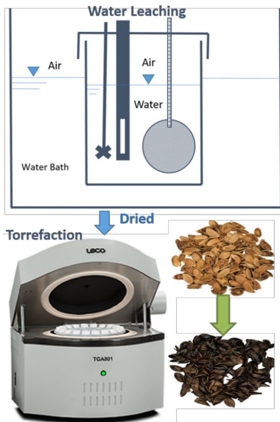
Figure 9. Laboratory scale leaching and torrefaction test equipment.
