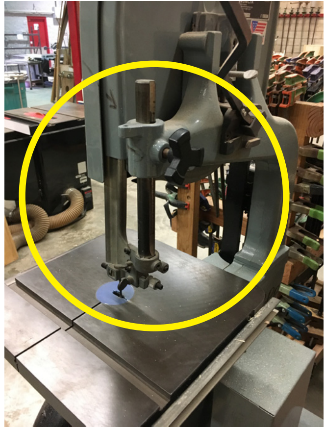
The guard can be found on the back of the bandsaw. Adjust it so it sits 1/2" above your stock.
